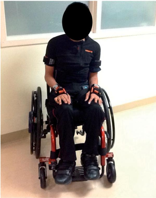
Figure 1. Participant and wheelchair setup, showing IMU sensors and instrumented pushrim. The supplied elastic straps, tight Lycra™ suit top and gloves were used to fix the sensors according to the system manufacturer's protocol.
